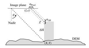
Figure 3. Measurement of height differences
